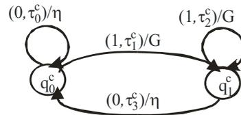
Figure 1. Input/output signal processing by the cellular biosensor modeled by  $TT_c$ .
