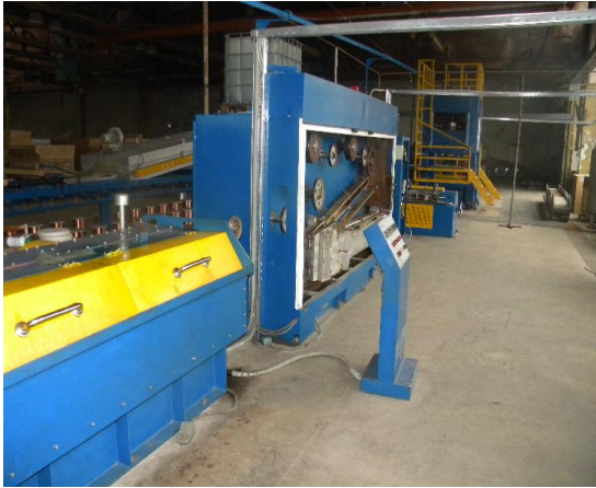
Fig. 7 General view of wire drawing line with annealing module
