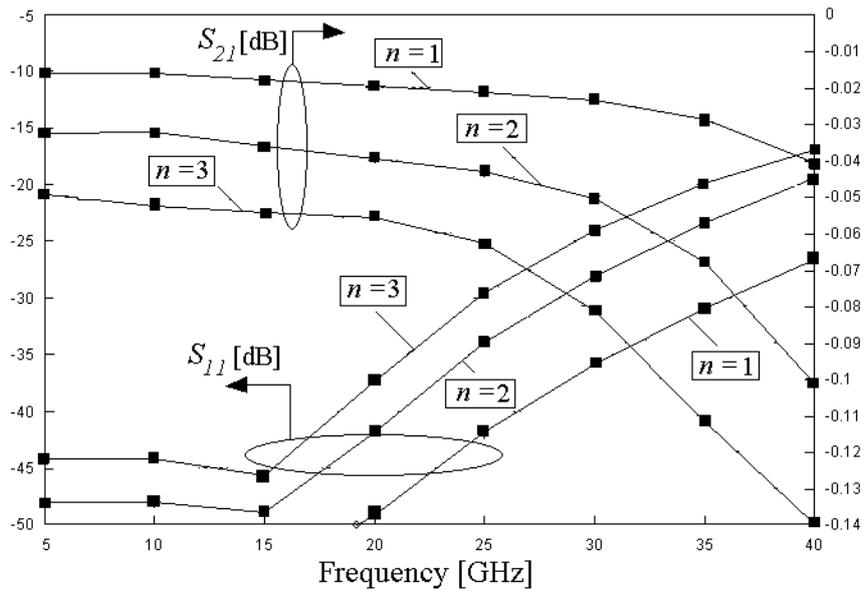
Fig. 3:  $S_{21}$  and  $S_{11}$  versus the frequency, for the MEMS switch designed in this paper.
