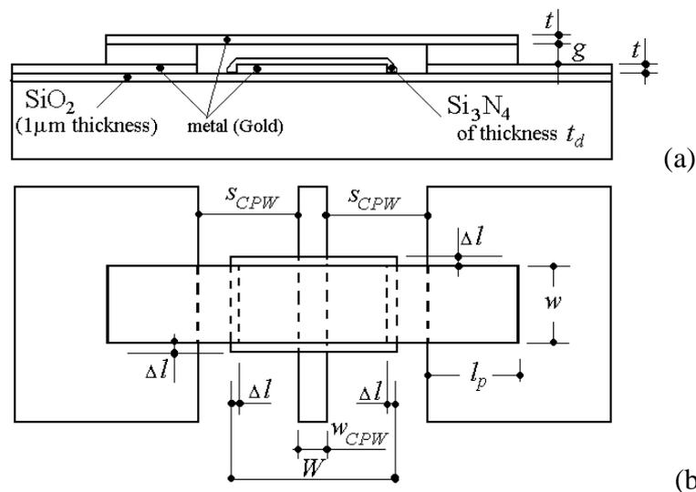
Fig. 2: The cross section (a) and the top view (b) for the MEMS used in this paper.
