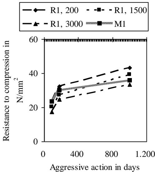
Figure 1. The variation of resistance at compression for recipe 1 in magnesian corrosion condition, 200, 1500 and 3000 mg/dm<sup>3</sup>.
