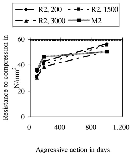
**Figure 3.** The variation of resistance at compression for recipe 3 in magnesian corrosion condition, 200, 1500 and 3000 mg/dm<sup>3</sup>
