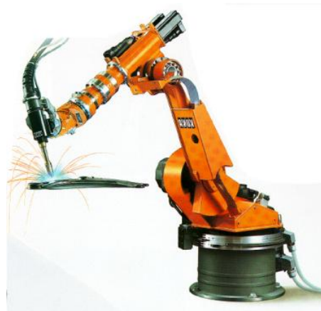
Fig.1 Robot Industrial in operatii de sudare
