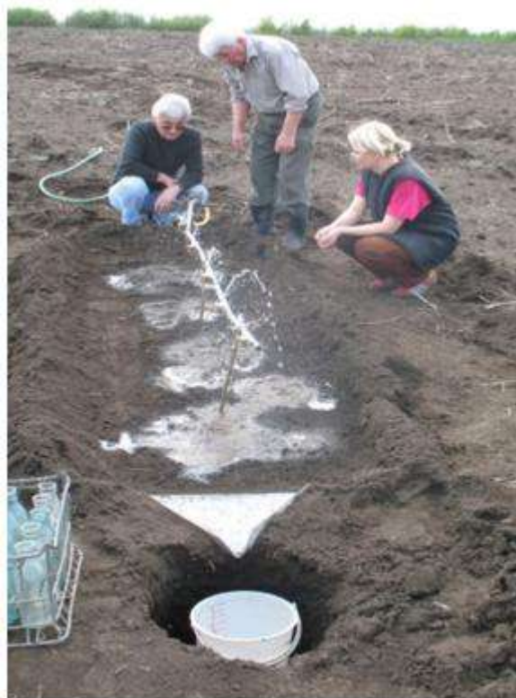
Figure 3. Determination of volume and turbidity of leakages under artificial influence of certain intensity [4]
