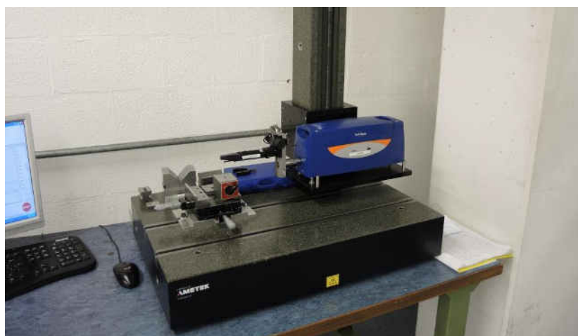
Figure 4. Measurement of surface roughness using Form Talysurf 50 (Taylor Hobson Co Ltd).
