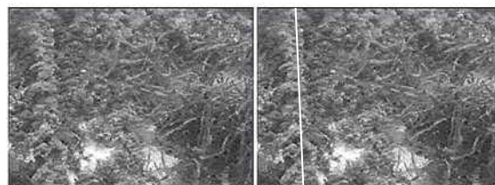
Fig. 3 (left) Original image of the cable; (right) evaluation of the cable (light line) after processing the original image.
