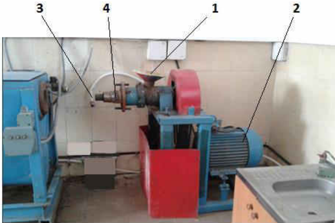
Fig. 1. Single-screw conveyer extruder for grinding maize and rape straw: 1 – loading throat; 2 – electric motor; 3 – die; 4 - screw conveyer
