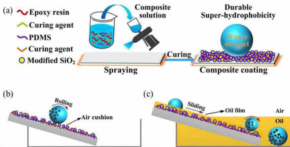
Figure 1. Schematic diagram of a spray-coating process
