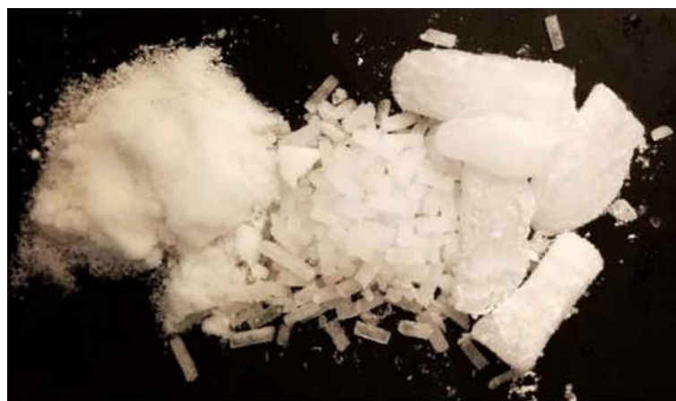
Figure 5. Dry ice, from left to right: loose, 3 mm pellets, 16 mm pellets [16]
