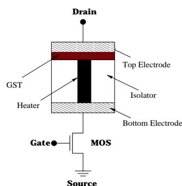
Figure 1: Cross Section of PCM Cell
