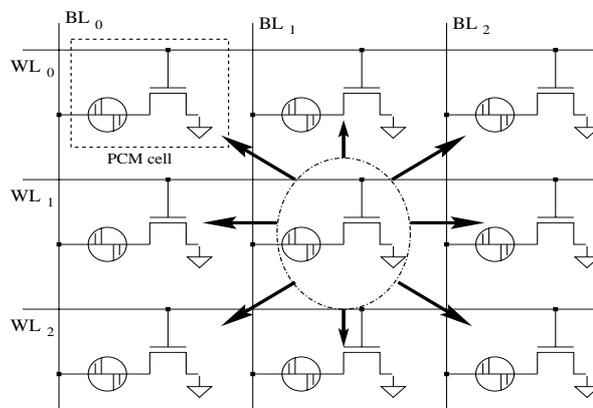
Figure 3: PCM Memory Array
