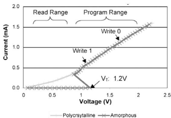
Figure 2: IV Characteristics of PCM Cell [10]
