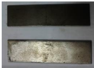
Fig. 2.3. Epruvete experimentale 100x26x2mm
