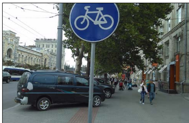
Figure 6. Bicycle lane laid out on sidewalks, in the form of a strip of pavement of a different color [31].
