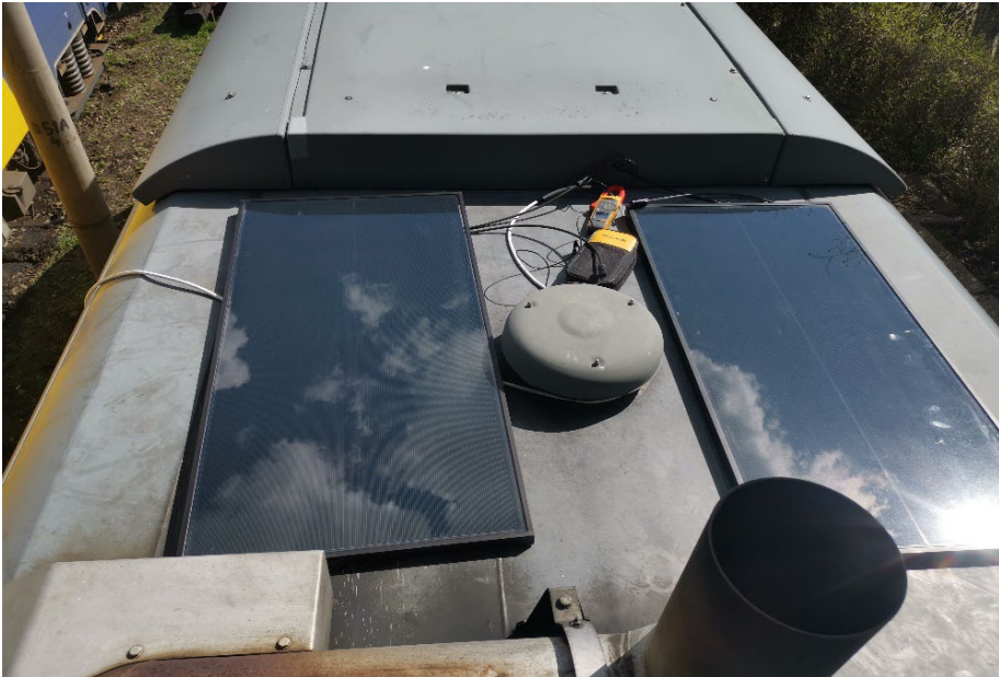
Fig. 5. View with photovoltaic panels placed on the roof.
