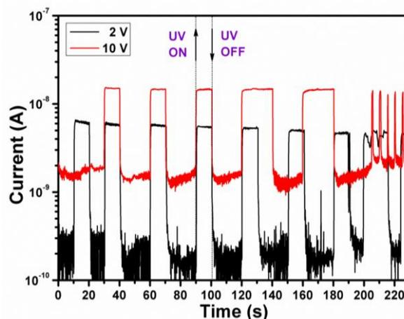
**Figure 2.** UV response of TiO<sub>2</sub> thin films with 15 nm with Ag-functionalized surface at two different applied bias voltages as 2 V and 10 V, respectively.
