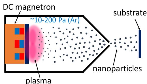
**Figure 1.** Schematic drawing of the gas aggregation source used for deposition of nanoparticles.
