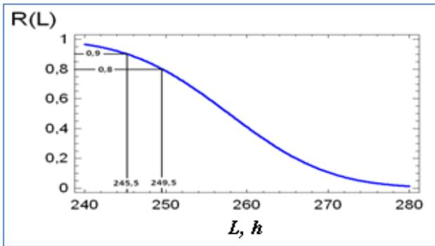
**Figure 5.** Sustainability percentage range of 80 to 90% of metallpolimers Ø40H8/e7 joints tested under dry friction: *Conditions: accelerated tests under cyclic oscillating,  $p = 3,5 \text{ MPa}$ ,  $n = 1800 \text{ min}^{-1}$  ( $v = 3.8 \text{ m/s}$ ), measurements were carried out at parts temperature of  $20 \pm 2^\circ\text{C}$  and air relative humidity of 60 ... 70%.*
