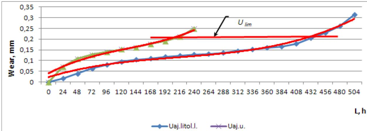
**Figure 4.** Evolution of wear of tribological co couplings adjustment Ø40H8/e7 tested under dry friction and boundary lubrication with LITOL24 STAS 21150-87: Test conditions: accelerated tests under cyclic oscillating regime,  $p = 3,5 \text{ MPa}$ ,  $n = 1800 \text{ min}^{-1}$  ( $v = 3,8 \text{ m / s}$ , the measurements were carried out at parts temperature of  $20 \pm 2^\circ\text{C}$  and air relative humidity 60 ... 70%.
