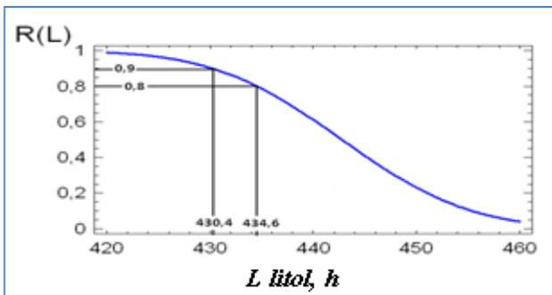
**Figure 6.** Sustainability percentage range of 80 to 90% of metallpolimers couplings Ø40H8/e7 tested under boundary lubrication with LITOL24:
