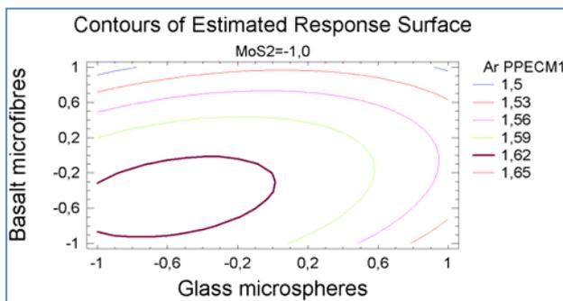
**Figure 2.** Estimating the relative adhesion of the PCM of polyamideepoxy matrix by reference of the concentration of the constituents (for the case of Mo concentration of disulfide 1 (code) 1% (real).
