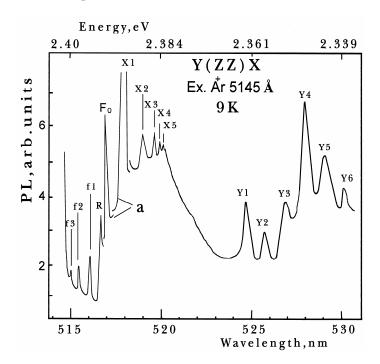
Fig.1 Luminescence spectra of CuGaS<sub>2</sub> crystals at 9 K excited by line 5145 Å of argon laser.
