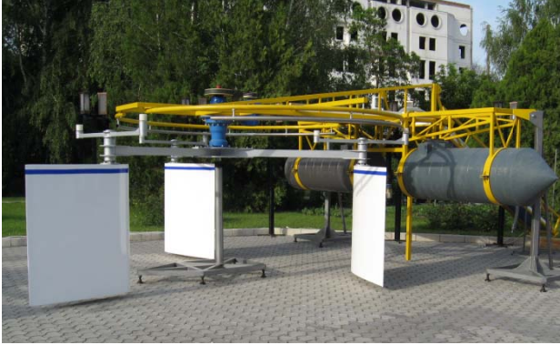
Figure 1. Micro-hydro power station with 3 hydrodynamic blades.
