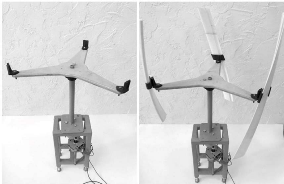
Figure 9. Changing the blades allows forming different VAWTs with the same tower supporting arms and electric generator.
