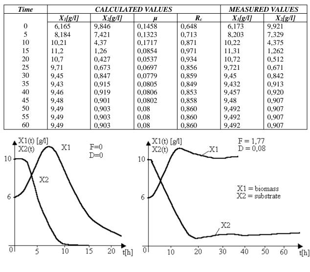
**Figure 1.** The calculator simulation results for the case of the discontinuous process (a), and for the case of the continuous flow process (b).
