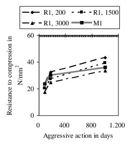
**Figure 1.** The variation of resistance at compression for recipe 1 in magnesian corrosion condition, 200, 1500 and  $3000 \text{ mg/dm}^3$ .
