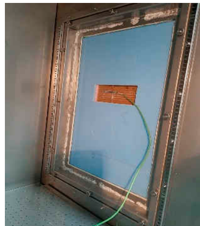
Climate chamber no. 1—hot face Temperature sensor
