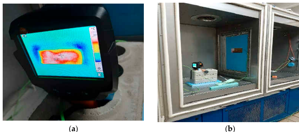
Figure 7. Thermographic test preparation in a double climate chamber. (a) Thermal image of sample no. 1; (b) Double climate chamber—test preparation.
