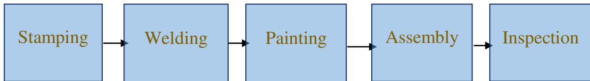
Figure 2. The flowchart of the manufacturing process [3]
