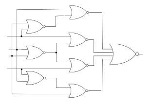
Fig. 1 Digital Circuit of Schneider counterexample
