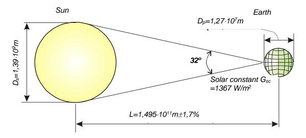
Figure 5. Geometry of the "sun-earth" system.
