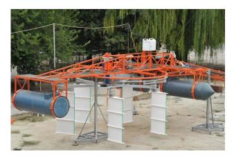
*Figure 12.* Microhydropower station for the river kinetic energy conversion into electrical and mechanical energies.
