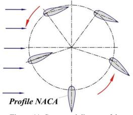
**Figure 11.** Conceptual diagram of the water rotor with hydrodynamic profile of blades with its orientation towards the water streams.
