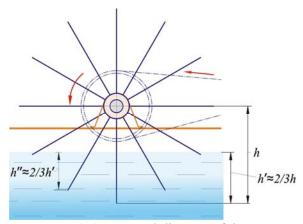
*Figure 10.* Conceptual diagram of the water wheel with rectilinear profile of blades.
