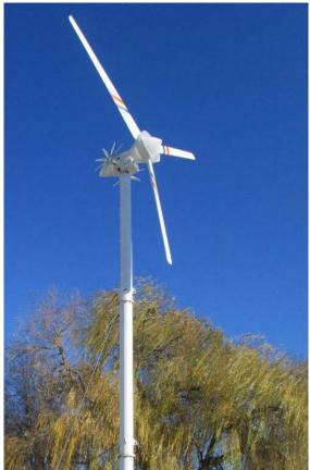
*Figure 14.* Wind turbine with mechanical orientation to the air currents.
