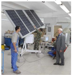
**Figure 9.** PV installation with orientation to the sun.
