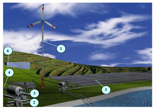
*Figure 15.* Drip irrigation system powered with electricity produced by the wind turbine.
