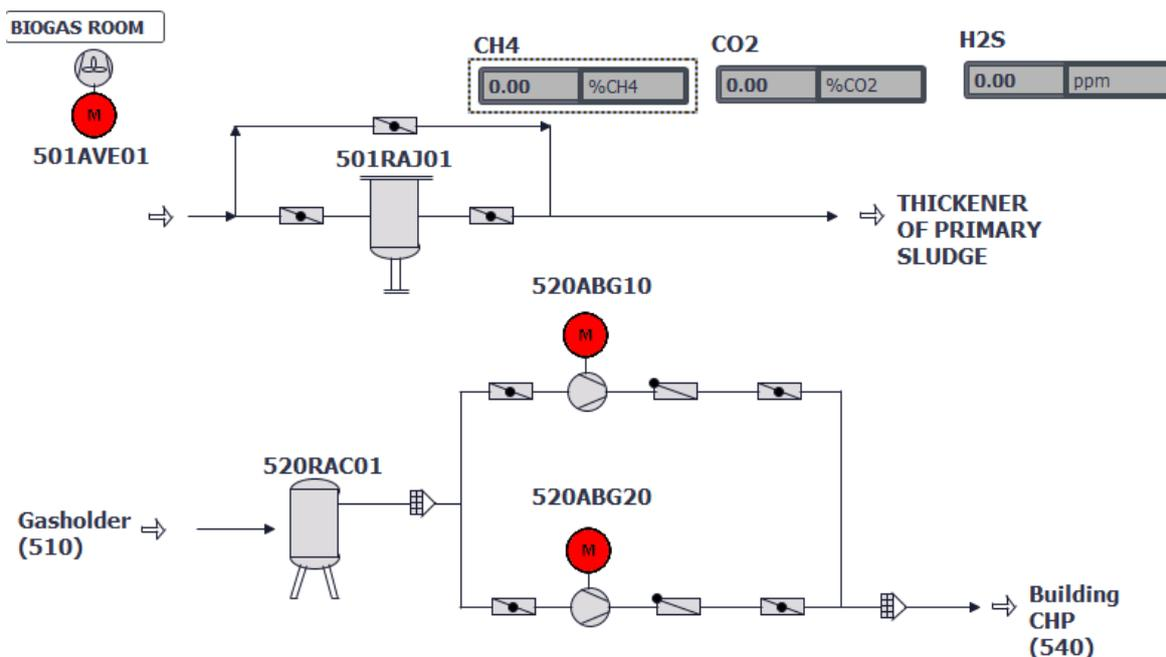
Figure 1. Biogas room [14].
