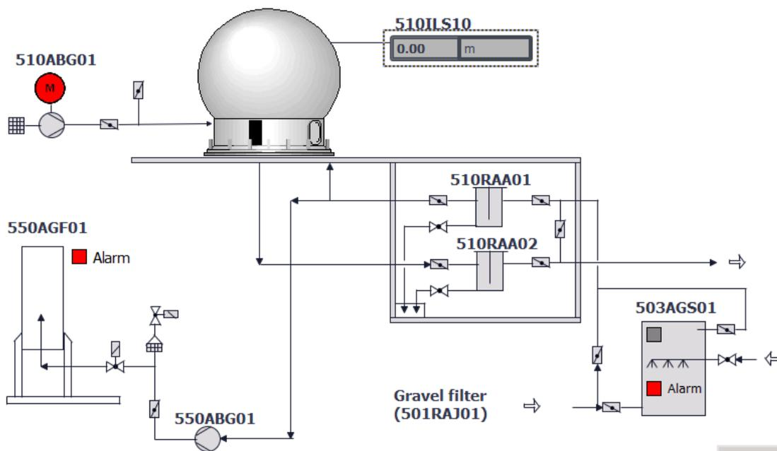
Figure 2. Desulphurization system, Biogas holder, Biogas flare [14].
