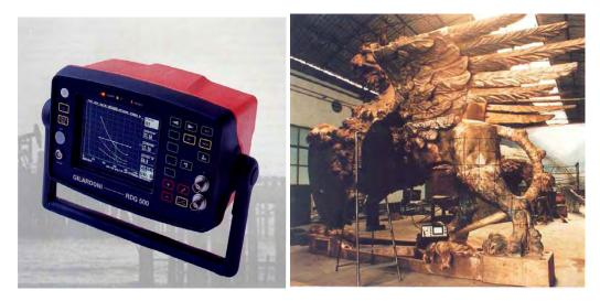
*Fig. 8.* The defectoscop type *RDG* 500 to control the layer state of preservation, thickness measurement, detection of hidden defects in metal, ceramic and marble sculptures.
