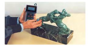
Fig. 9 The ultrasonic DG 40 B.
