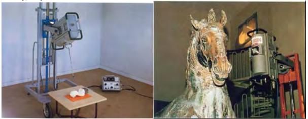
Fig. 6 Portable monoblock type MONOGIL MT 350/6 of roentgen ray for research of art objects made of metal, ceramic and stone. Sankt-Peterburg
