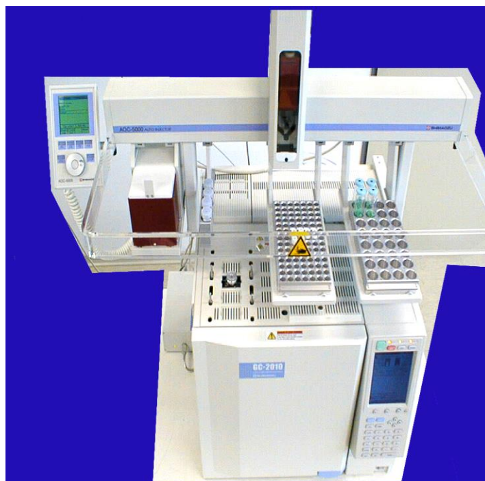
Fig. 1. GC/MS QP2010SE coupled with three-dimensional automated system for sample injection AOC-5000
