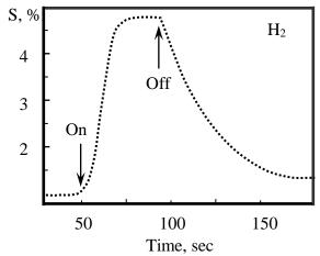
Figure 3. Gas sensitivity of single nanorod-based sensor.
