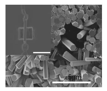
Figure 2. SEM images of silver-doped ZnO nanorods. Inset show an individual nanorod-based sensor fabricated by nanolithography in focused ion beam system. Scale bar is  $5 \mu m$ .
