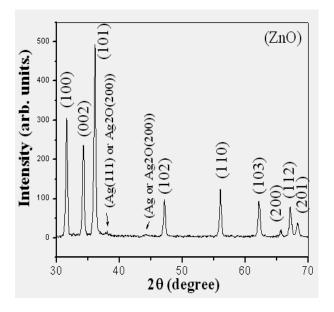
Figure 1. The XRD pattern of the ZnO nanorods.
