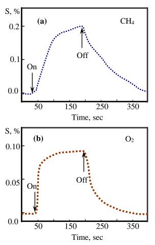
Figure 4. Gas sensitivity of single nanorod-based sensor to (a)  $CH_4$  and (b)  $O_2$  gases at room temperature.
