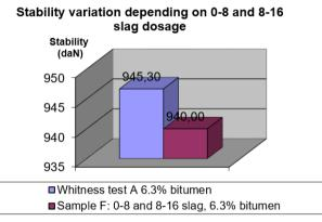
**Figure 4.** Comparison between Marshall stability obtained on control and 0-8+8-16 slag samples.
