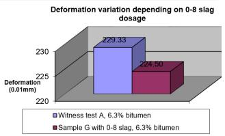
**Figure 2.** Comparison between the flow index determined on control and 0-8 slag samples.
