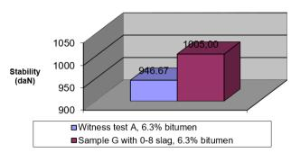
Figure 1. Comparison between Marshall stability determined on control and 0-8 slag samples.
