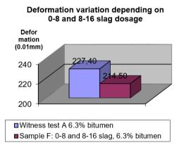
**Figure 5.** Comparison between the flow index determined on control and 0-8+8-16 slag samples.
