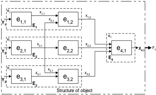
**Figure 2.** Functional and diagnostic model of the object, where:  $E_i$  –  $i^{\text{th}}$  functional assembly in the object,  $e_i - j^{\text{th}}$  subassembly or functional element in a given assembly,  $Y_{1,2,3}$  – input signals in the object
