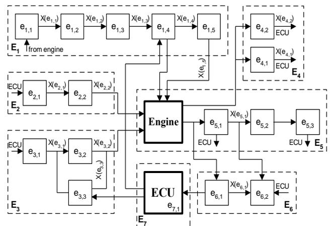
**Figure 4.** Diagram of an electronic controller for an automotive engine, where:  $E_1$  – ignition module,  $E_2$  – fuelling module,  $E_3$  – air-feeding module,  $E_4$  – starting circuit,  $E_5$  – power supply circuit,  $E_6$  – engine block,  $E_7$  – electronic control unit
