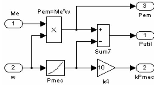
Figure 5. Model of output power
