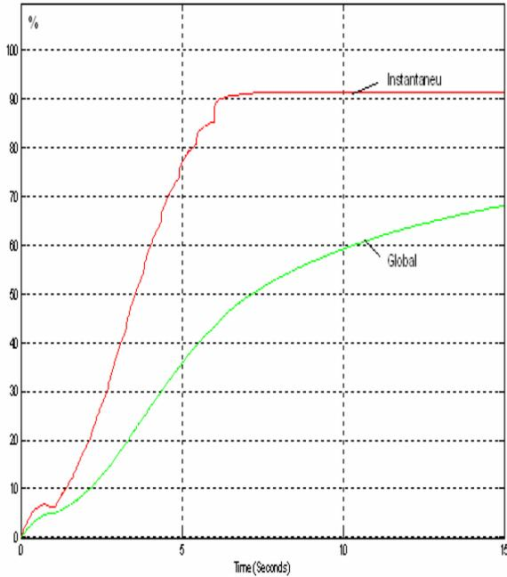
Fig.9 Instantaneous and global efficiency
