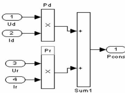
Figure 4. Model of power consumption
