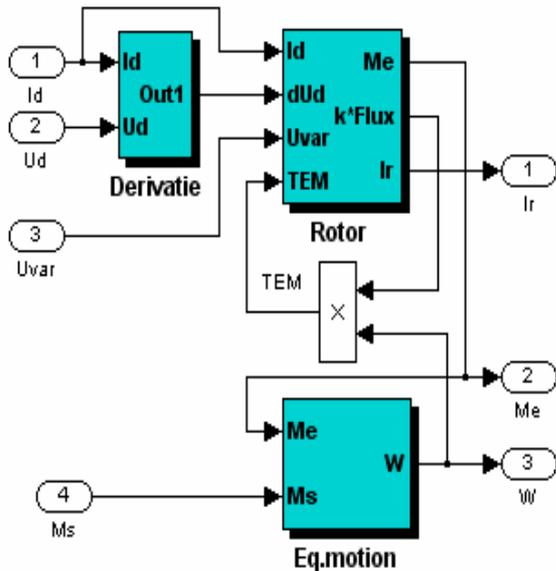
Figure 3. Model of Compound DC Motor
