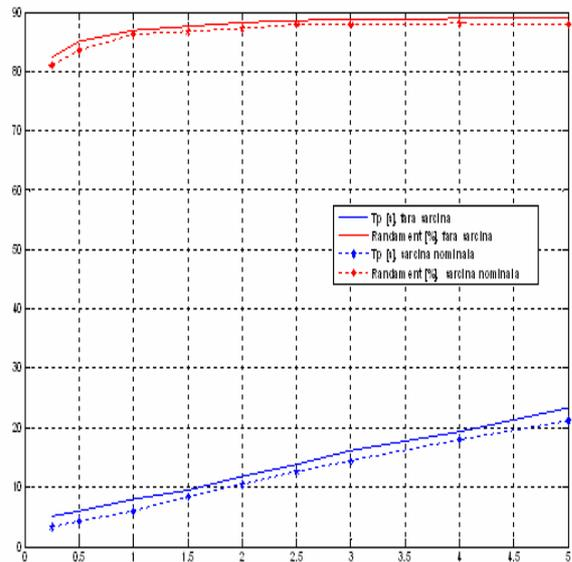
Fig.14. Dependens  $T_p$ , Randament= $f(t_{comuat})$
