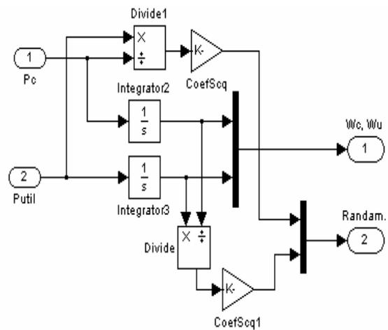
Figure 6. Model of output power
