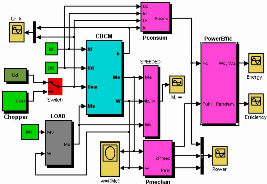
Figure 2. Mathematical model of trolleybus traction
