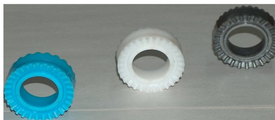
Fig. 4. Satellite gear wheels cast from different plastic materials
