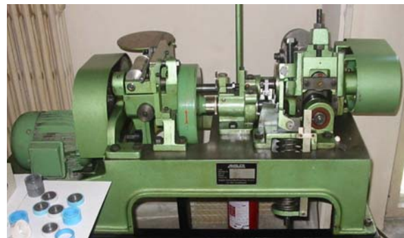
Fig. 5. Laboratory installation „Amsler A 135”
