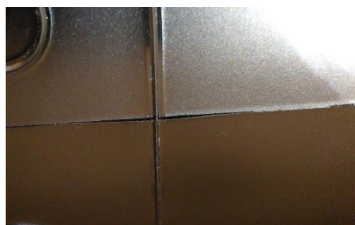
Fig. 10. New, non-conforming die cut. The die cut overlaps when mounted, causing the material to cut/tear.
