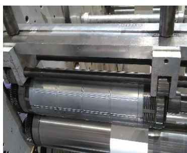
Fig. 6. Die cutting a width of material narrower than the die itself wears out the die.
