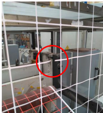
Fig. 4. The waste matrix is broken.
