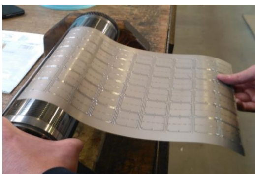
Fig. 1. The die is flat-shaped. It is mounted on the magnetic cylinder by rolling.
