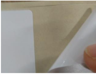
Fig. 11. The die does not correctly cut the face of the material.
