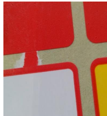
Fig. 5. Incompletely cut labels that remain attached.
