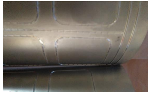
Fig. 15. Matching die cuts independently executed. Checking the nest overlap is done by matching the die cuts at the edge.
