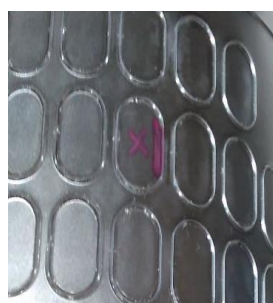
Fig. 7. Die cut with a partially destroyed nest – see the "X" red mark.
