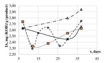
A) Dynamics of spread acidity index (IA), 3.5 being maximum acceptable limit (MAL)
