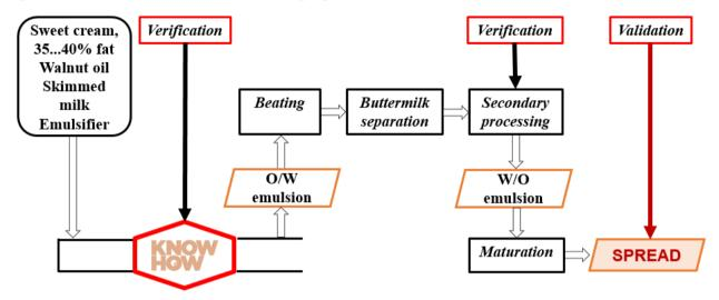
Fig.12. General scheme of the spread manufacturing process according to the invention patent, No. 1281, 2018.09.30.
