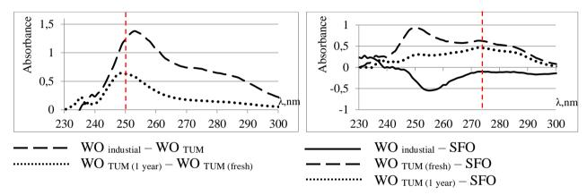
Fig.4. Differences between the spectra of walnut oils (1:80 dilution, solvent and reference - chloroform)
