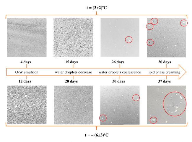
Fig.16. The aggregative stability of the microstructure of spread containing walnut oil
