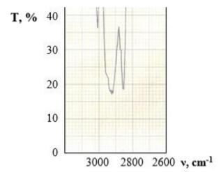
Fig.2. Fragment of the IR spectrum of the WO freshly pressed: valence oscillations of C-H bonds
