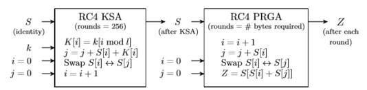
Figure 1: Description of RC4 stream cipher [5]
